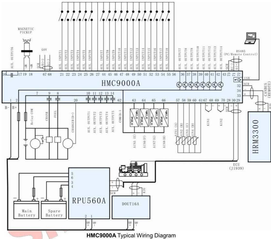
**HMC9000A Typical Wiring Diagram**
